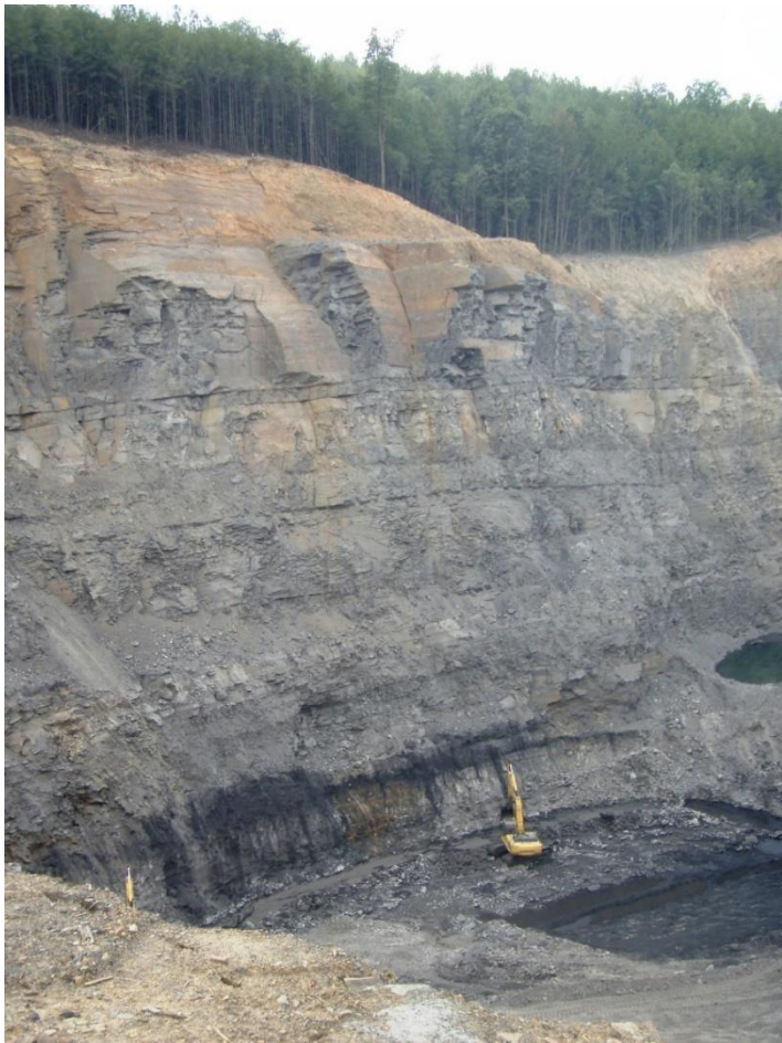
Figure 5. This view shows the whole section of coal seams. From the bottom: Jagger, Blue Creek (the thick seam), Mary Lee, Lower Newcastle, and Upper Newcastle. Photo courtesy of Bill Lawrence.
