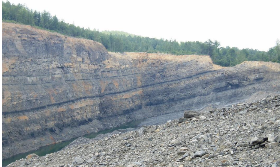
Figure 4. View of the coal seams at the RJR coal mine: from the bottom, Jagger, Blue Creek (the thick seam), Mary Lee, Lower Newcastle, and Upper Newcastle. Photo courtesy of Bill Lawrence.
